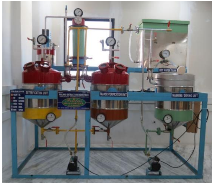
50 litres Biodiesel Plant at Centre for Waste Management operated since April 2015
