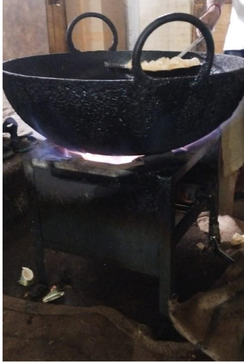
Biogas fuelled Stove in the mess
