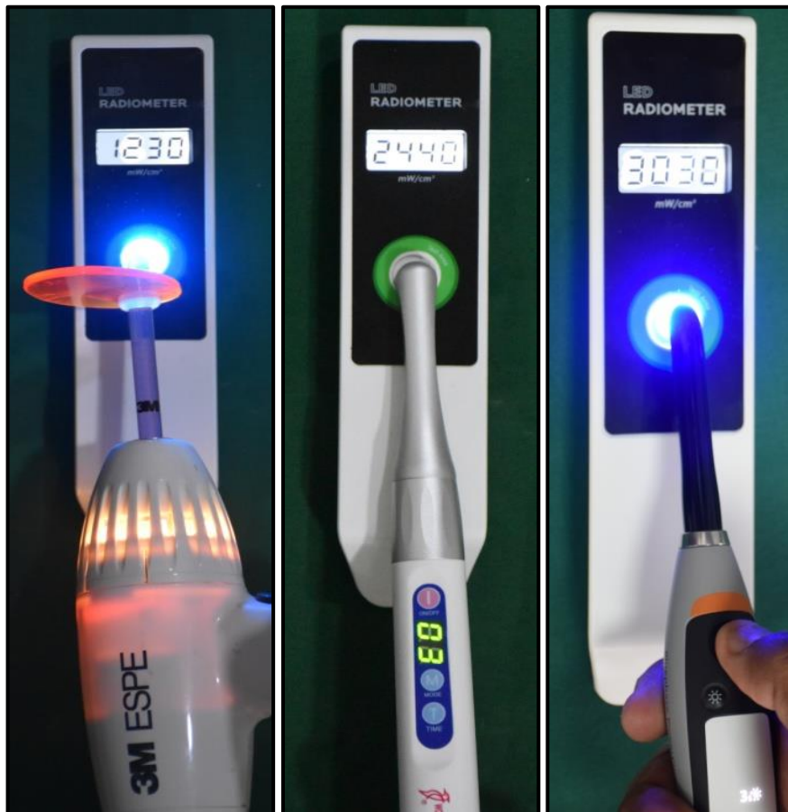
FIGURE 7: LIGHT INTENSITY TESTING USING BEHN-LED1
