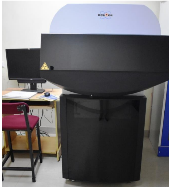
Figure 11: Bruker micro-CT machine (Sky scan 1176, Kartuizersweg 3B, Belgium)
