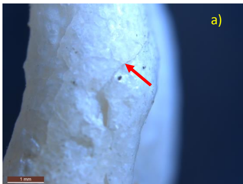
Figure 6a & 6b: Excluded samples (Red arrow indicate samples with cracks and fracture) after stereomicroscope evaluation
