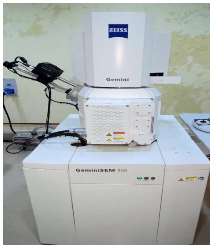
Figure 11: Scanning electron microscopy with X-ray energy dispersive mode. (Gemini SEM, Zeiss, Germany)
