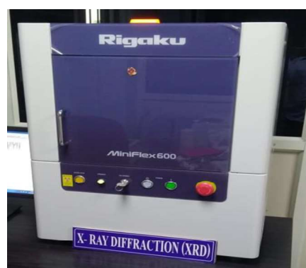
Figure 15: X – ray diffractometer (XRD) (Rigaku, Tokyo, Japan)
