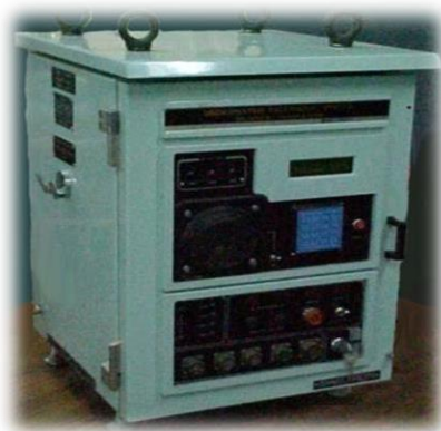
UNDER WATER TELEPHONE SYSTEM
