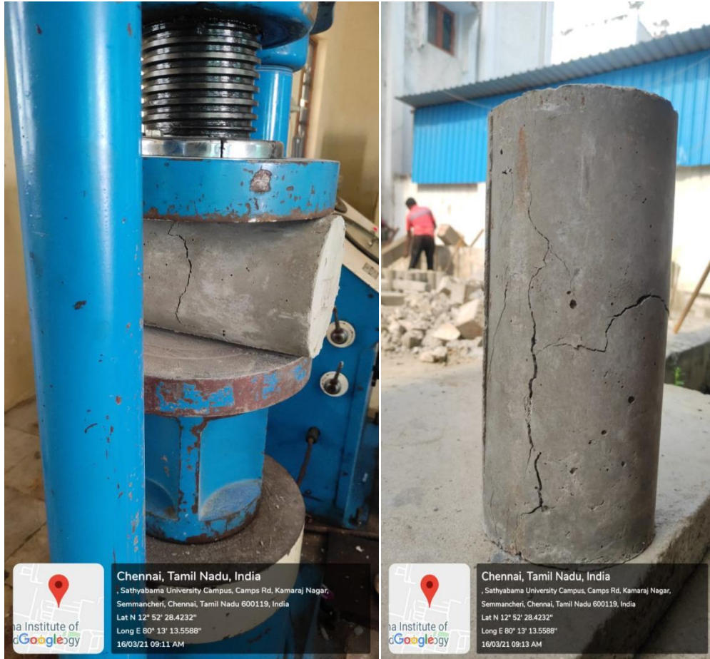
Fig. 4.10 Split tensile strength test
