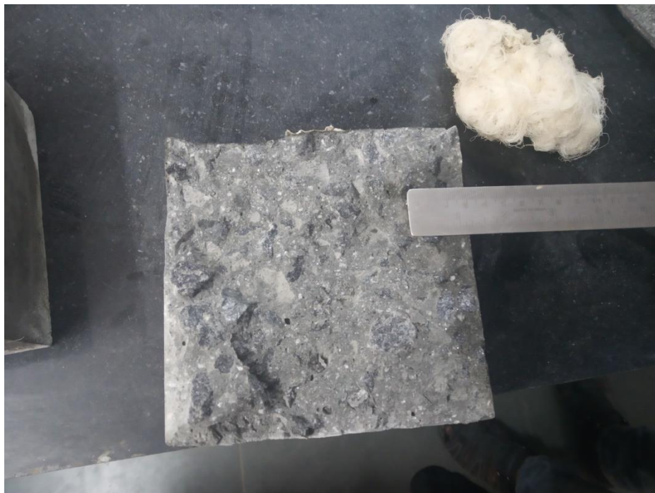
Fig 4.11 Measuring the depth of water penetration
