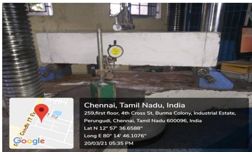
Fig 4.13 Beam subjected to three point loading
