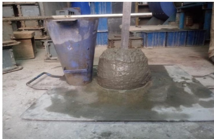
Fig 4.7 Measuring the slump of concrete
