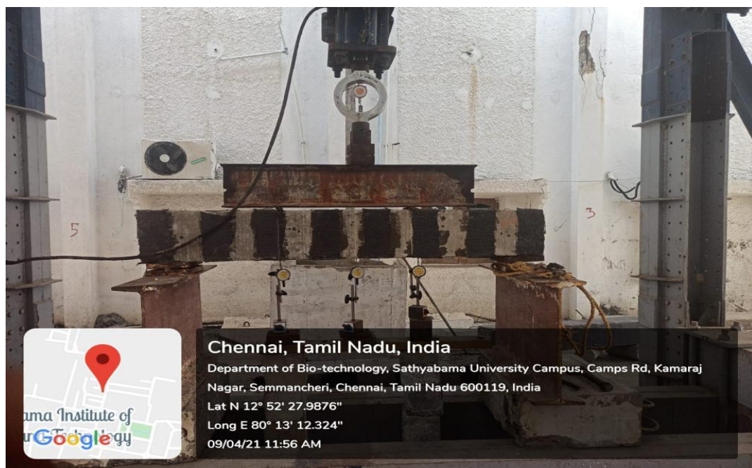
Fig 5.7 Experimental setup on CFRP wrapped beam with 100 mm interval
