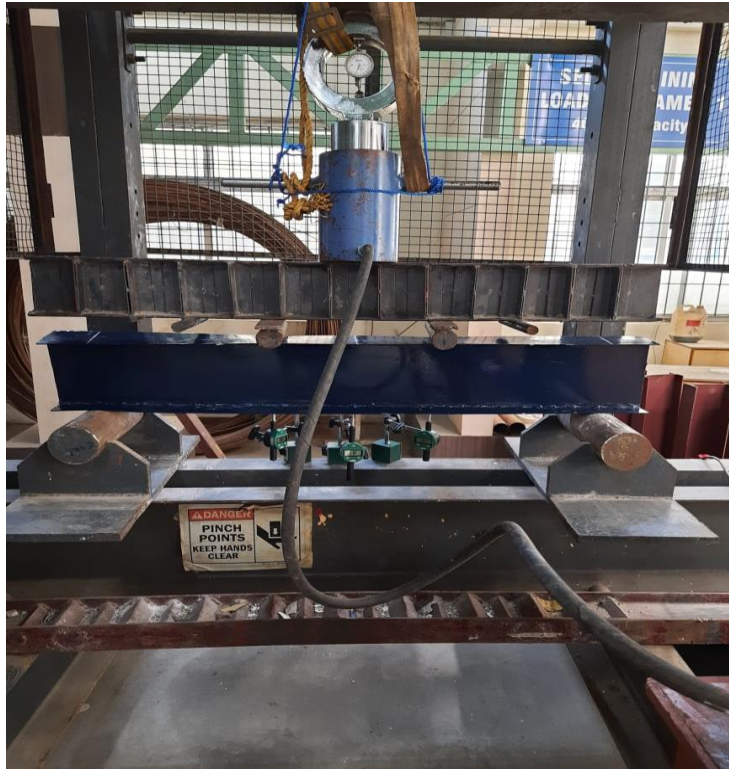
Fig 6.10: Testing Set-Up of CRB
