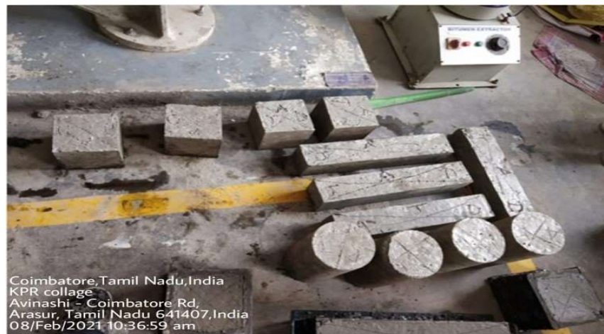
FIG 4.5 DEMOULDING OF CUBE, CYLINDER & PRISM
