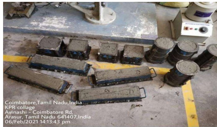
FIG 4.2 CASTING OF CUBE, CYLINDER & PRISM
