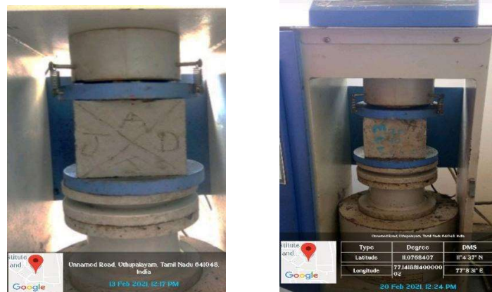
FIG 4.7 CUBE COMPRESSIVE STRENGTH TEST
