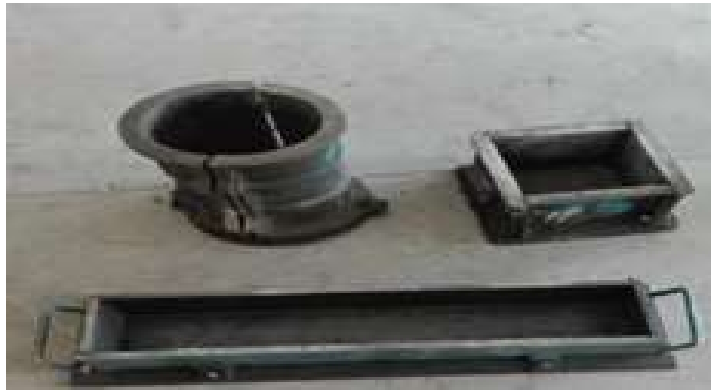
FIG 4.1 MOULD FOR CASTING OF SPECIMENS
