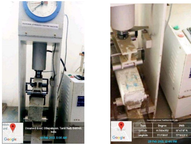
FIG 4.9 FLEXURAL STRENGTH TEST
