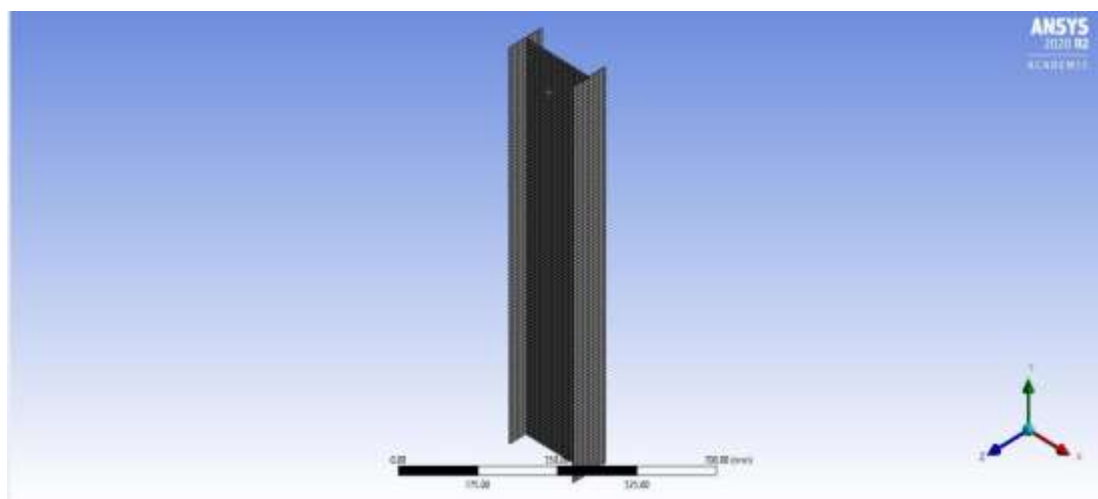
FIG5.6 MESHING OF BUILT UP I SECTION
