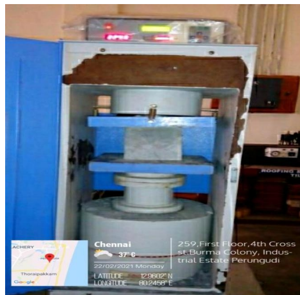
Fig 4.4 Cube Compression strength test
