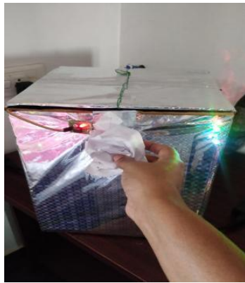
Fig.4. Completely filled dustbin with locking system ON (White, Green and Red LED is on HIGH)
