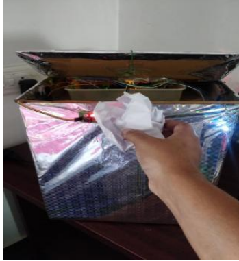
Fig.3. Not completely filled dustbin with locking system on OFF (White LED is on HIGH).
