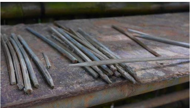
Use of Bamboo Nails for structural stability
