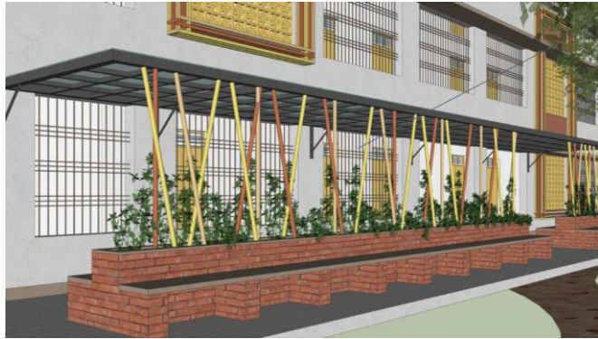
Additional Roof Canopy
