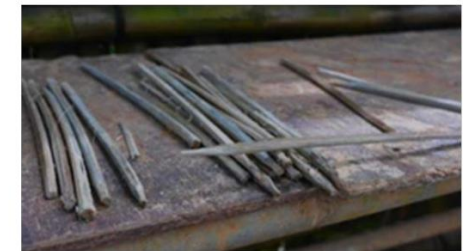
Use of Bamboo Nails for structural stability
