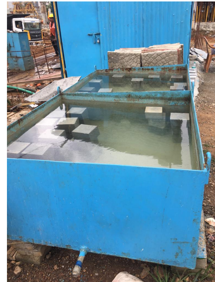
Fig 10 - RMC Mix - Curing of Cubes
