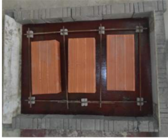
Fig 2.6 - Porotherm Bricks and Steel Bars
