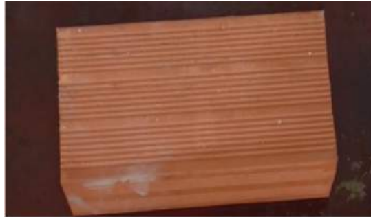
Fig 2.4 - Porotherm block of the size 400x100x200
