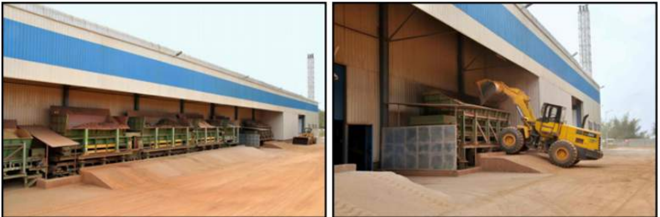
Fig 2.11 - Dosage of Raw Materials by Feeders
