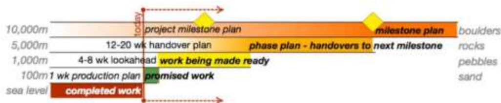
Fig 2.8 LPS Level of Detailing
