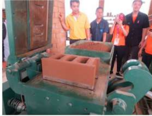
C. Block to be used for load bearing wall made from machine press
