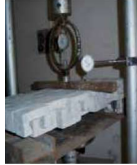
Fig 2.23 Setup for Flexural Loading Test
