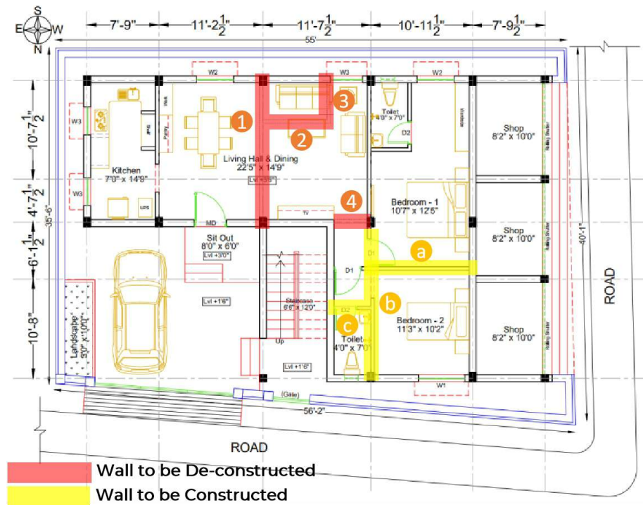
Fig 5.3 Walls to be de-constructed and re-constructed
