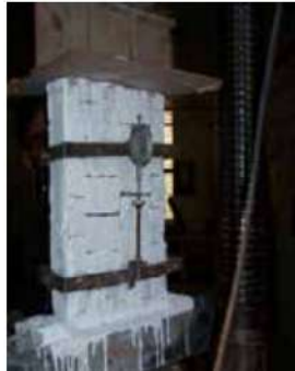
Fig 2.22 Setup for Compression Test
