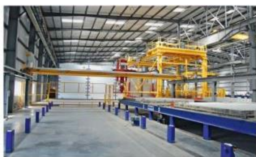
Special screeding lines with blade-equipped finishing heads ensure top architectural-concrete quality Figure: Vollert
