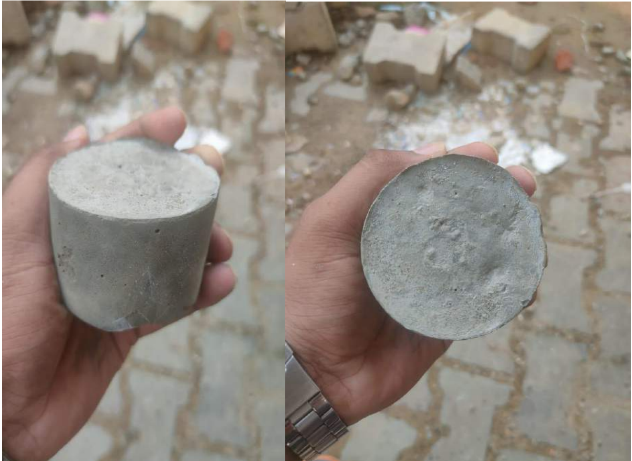
Fig 5.1 - Bioconcrete was demoulded
