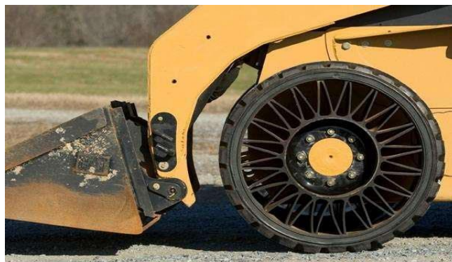
Fig:1.4 Airless Tyre Used In Earth Movers
