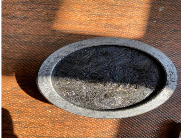
Fig:4.11: Composite material in die After heat press.
