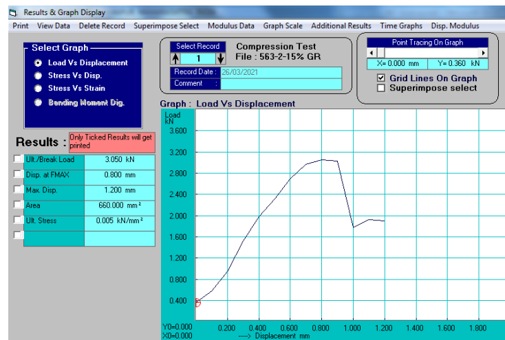
Fig. 5.20: Compression test of Sample 4 (14 days curing period)
