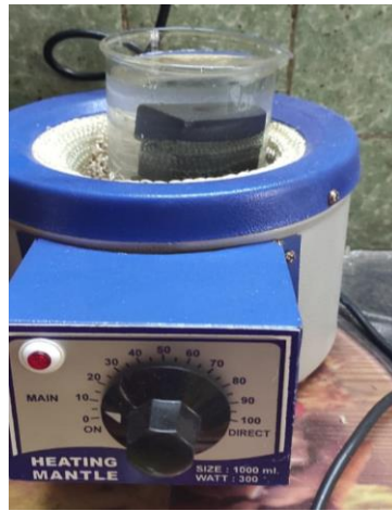
Fig: 5.27: Water absorption test experimental set-up
