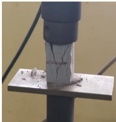
Fig: 5.21: Compression test experimental set-up
