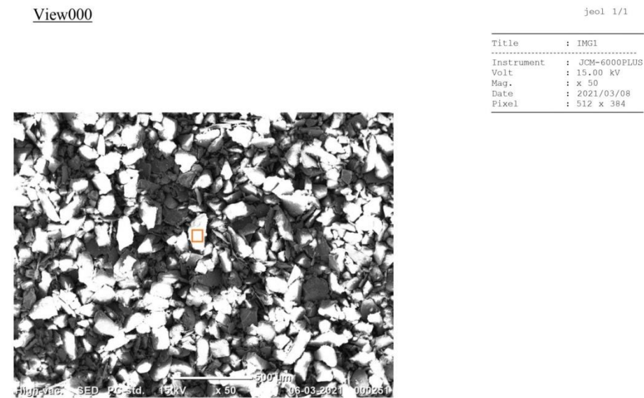
Fig. 5.7: River Sand SEM image (500µm)
