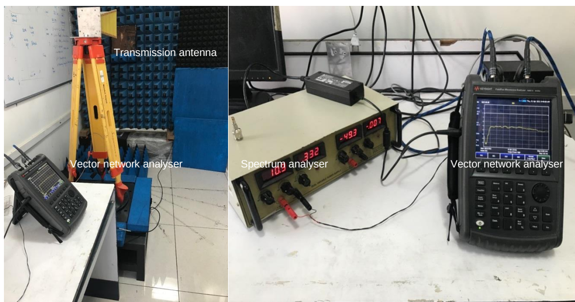
Fig: 5.36: Experimental set-up for VNA
