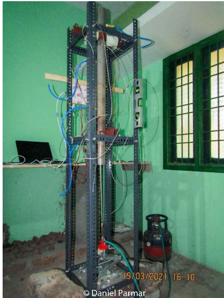
Fig 4.3 Rijke tube combustor containing electret microphones and thermocouples
