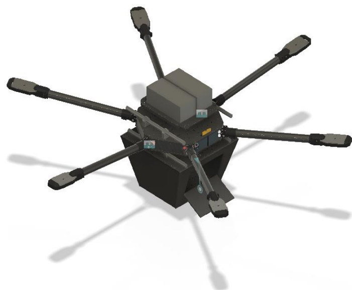
Fig 4.4.5 Full assembly with delivery payload
