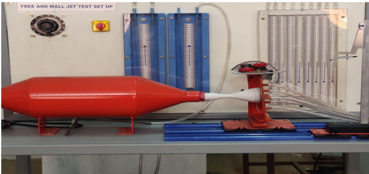
Fig. 5.2.3 Testing of a Cd Nozzle with Square Dimples in a Free and Wall Jet Test Set Up
