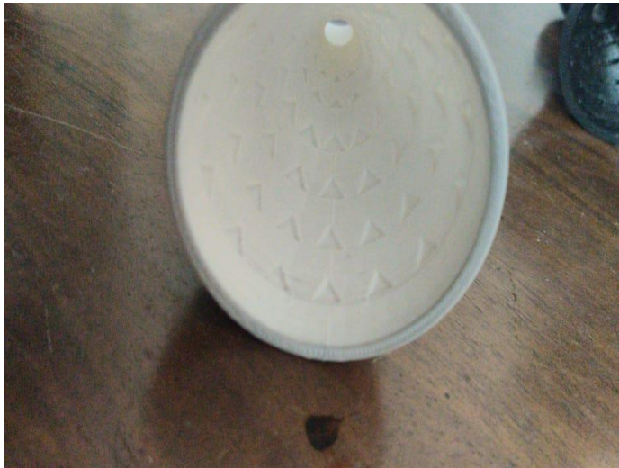
Fig. 5.1.1 Inner View of a Cd Nozzle with Triangular Dimples
