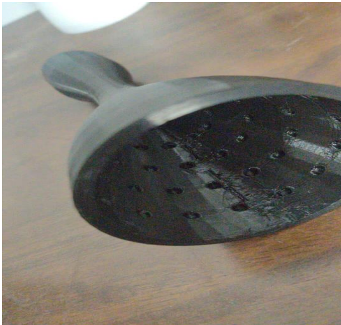
Fig. 5.1.2 Inner View of a Cd Nozzle with Circular Dimples
