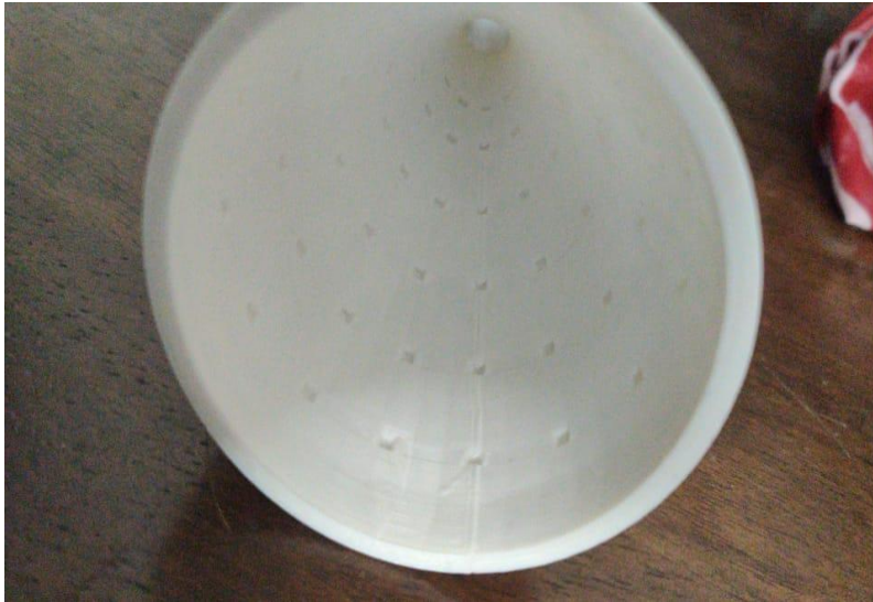
Fig. 5.1.3 Inner View of a Cd Nozzle with Square Dimples
