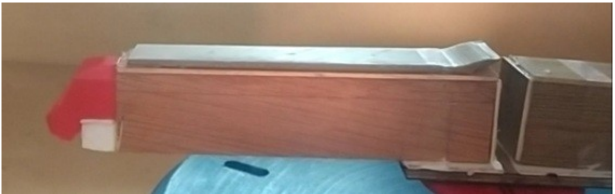
Fig 6.5 Modified fairings attached to the body of the model
