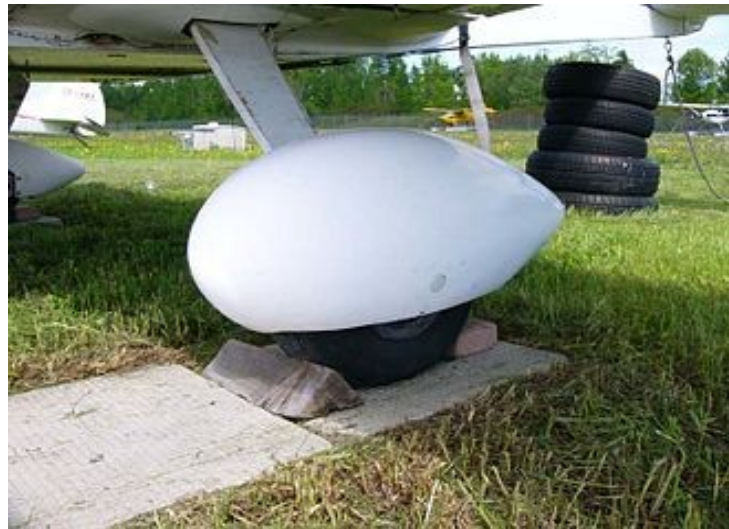
Fig 1.1 Aircraft wheel fairing
