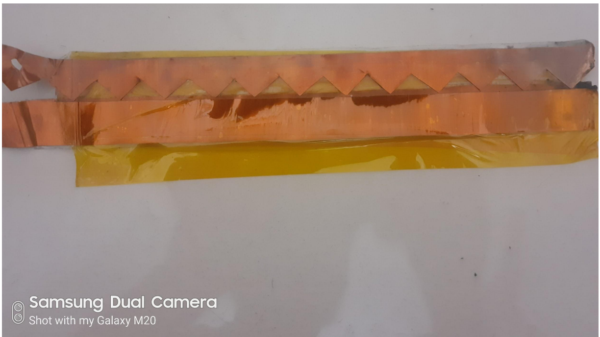
Fig No. 4.4 : Resulting manufactured DBD actuator with serrated electrode.
