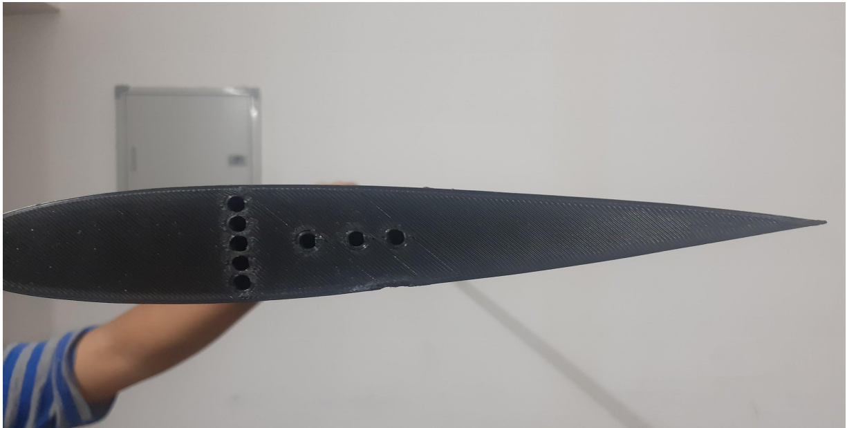
Fig No. 4.8 : Side View of the Airfoil : 8 Pressure Hole of 3mm diameter
