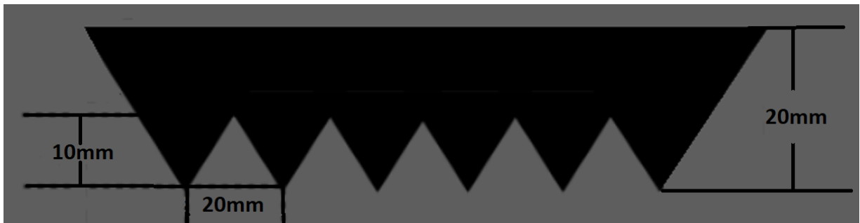
Fig No 4.2 : Dimensions of the exposed electrode
