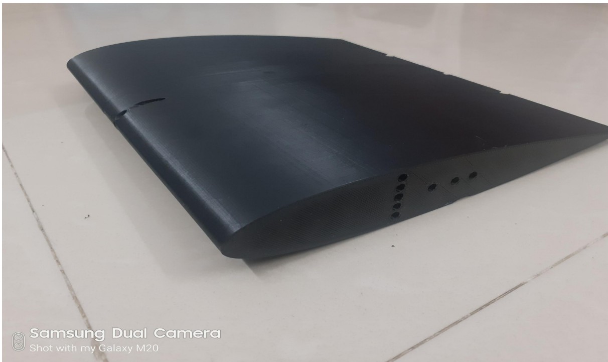
Fig No. 4.6 : 3D Printing of the airfoil
