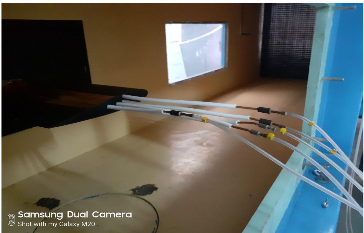
Fig No. 4.14 : Airfoil installed in test section
