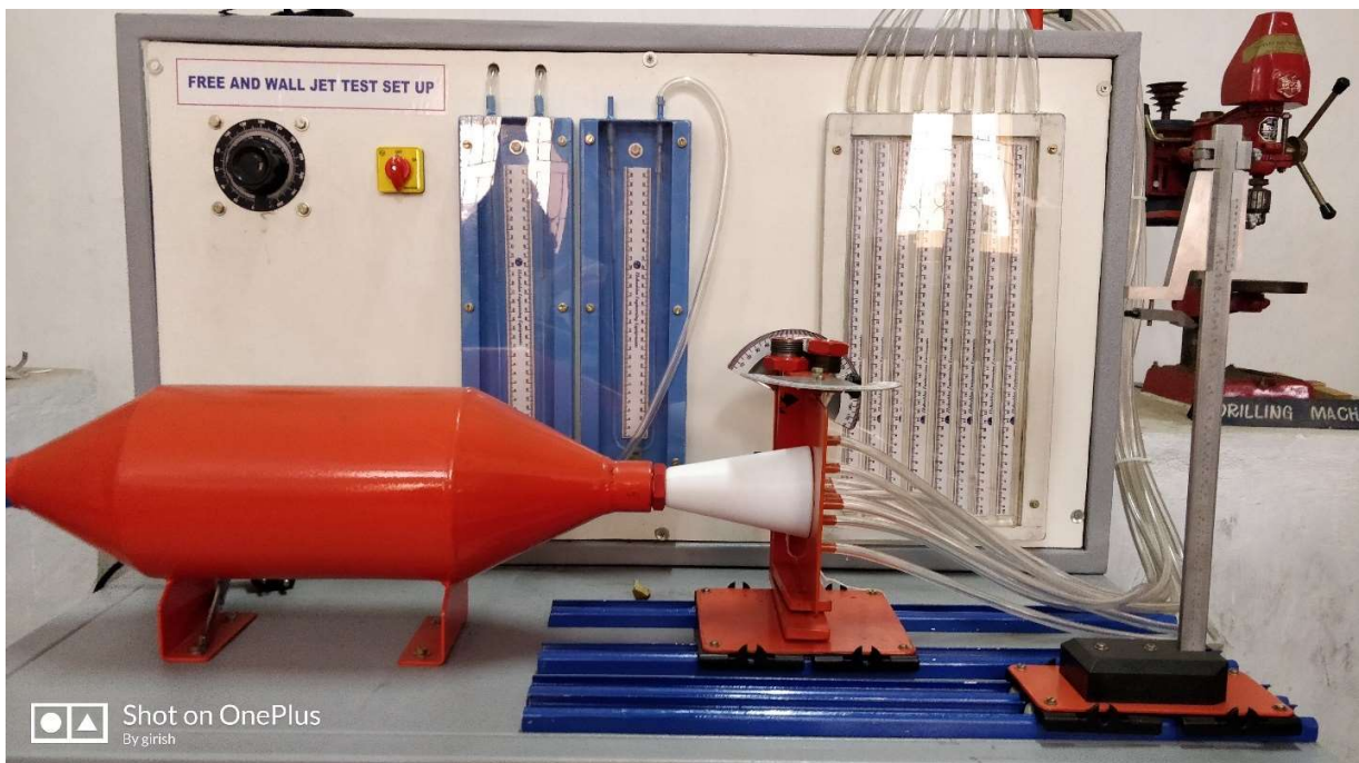
Fig No 4.3 Testing of Square CD Nozzle
