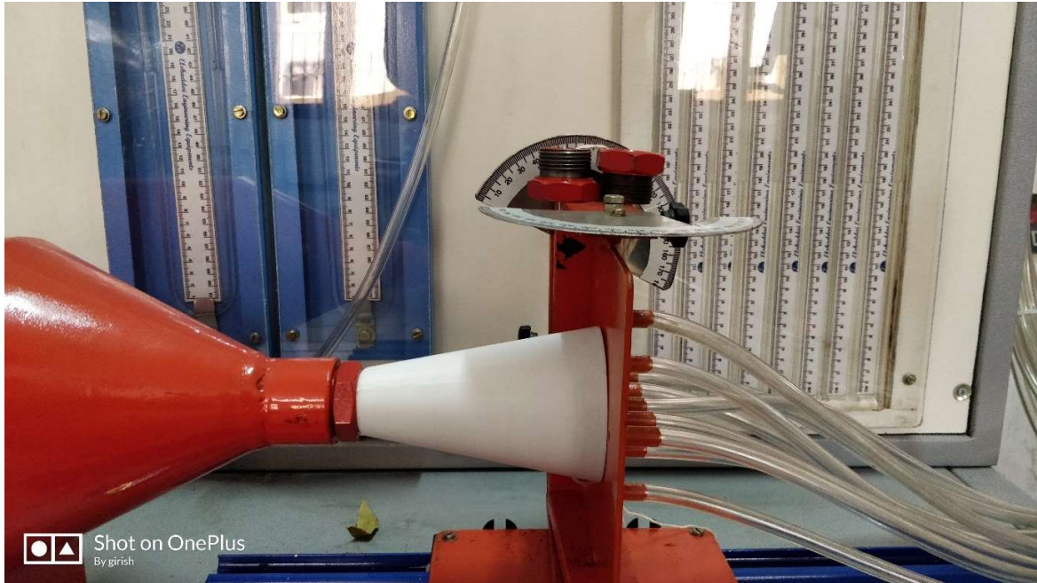
Fig No.4.2 Testing of Square CD Nozzle
