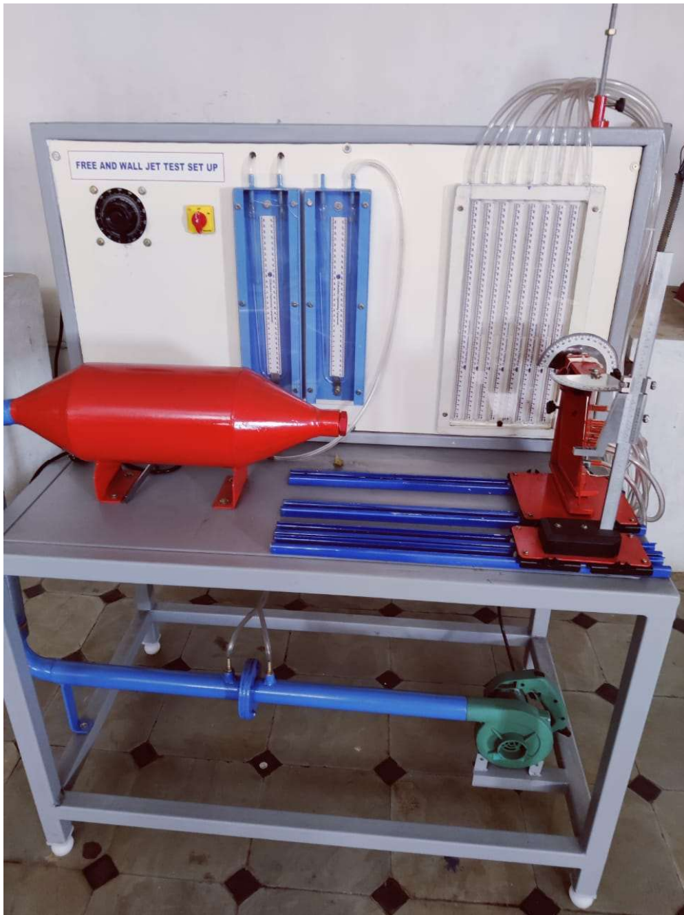
Fig No4.6 FREE AND WALL JET SET UP
