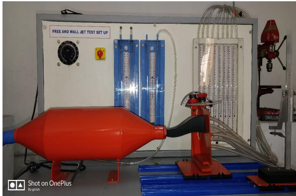
Testing of S Duct
