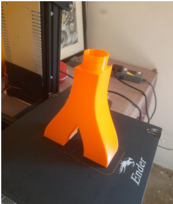
3D Design of Y Duct
