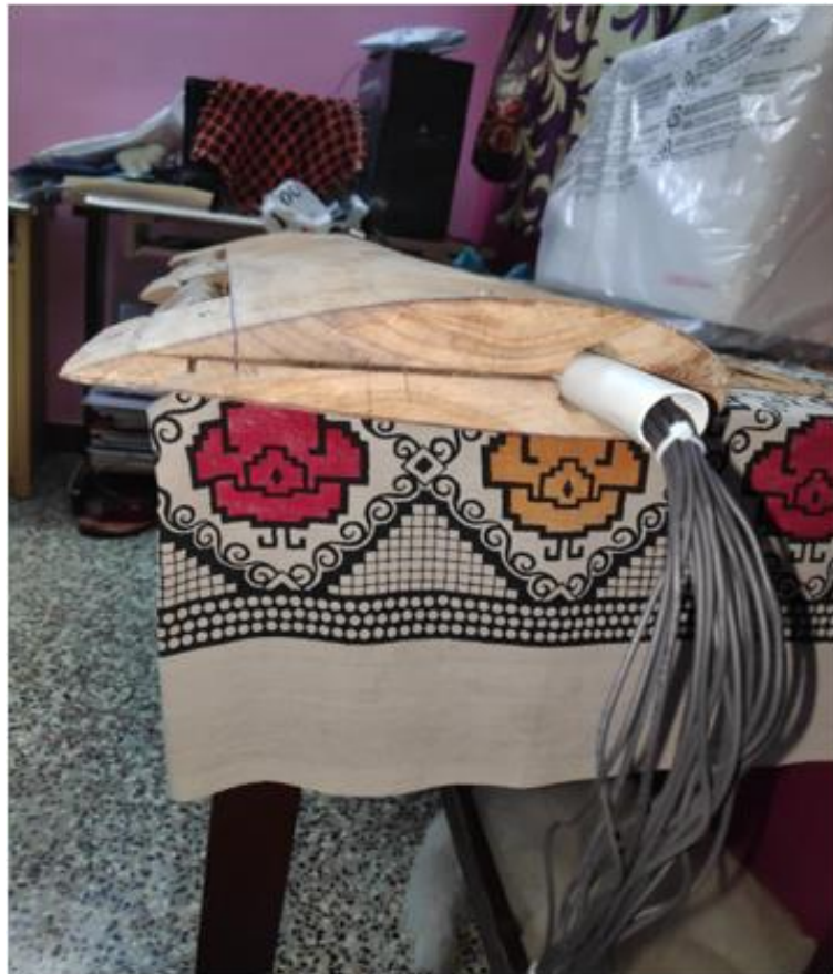
Fig 4.16 Side view - airfoil NACA 4418.
