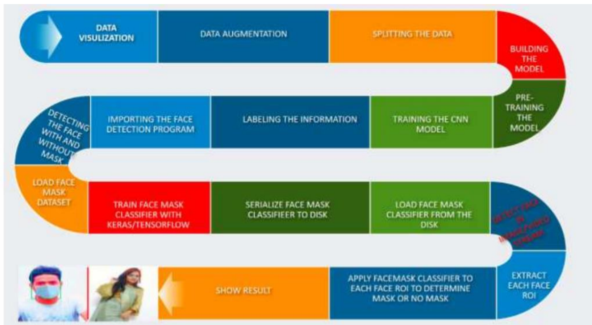
Figure 4.2: Flow diagram for face mask detection
