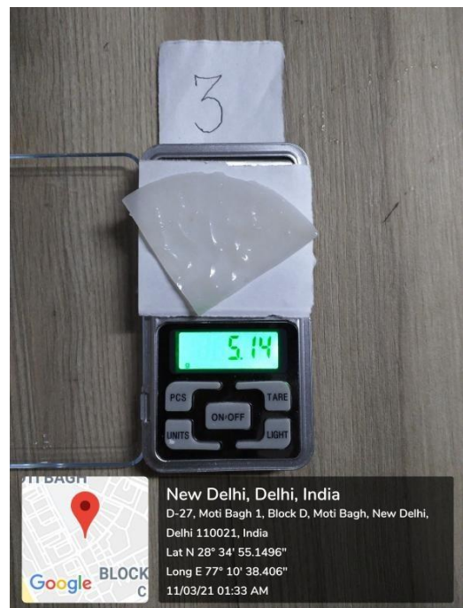
Fig:5.7 : Weight (in g) of the Bioplastics (Potato Starch) after 24 hours immersion in base
