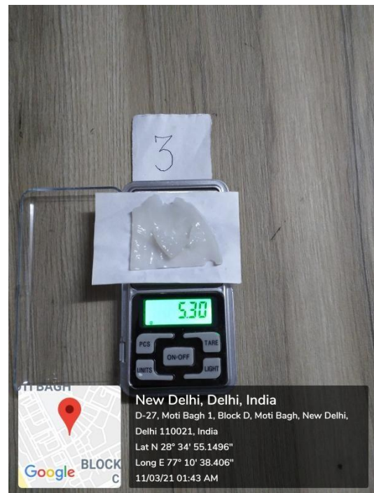
Fig:5.15 : Weight (in g) of the Bioplastics (Corn starch) after 24 hours immersion in base
