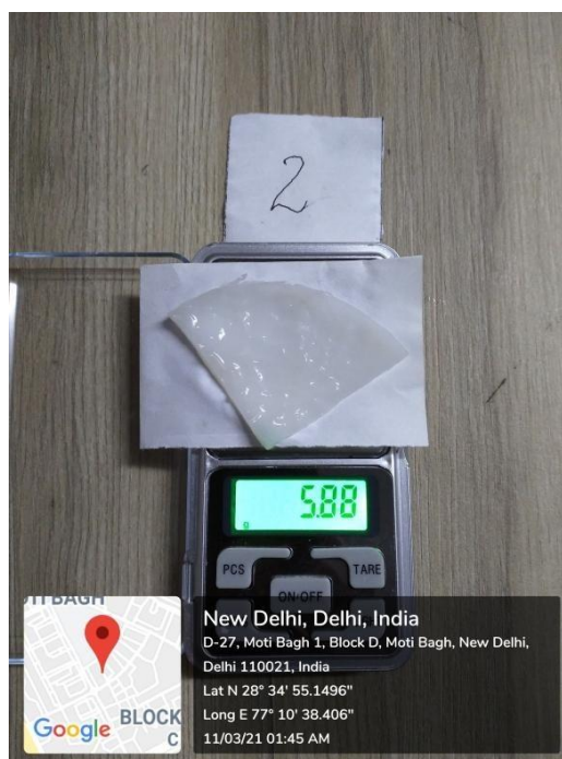
Fig:5.13 : Weight (in g) of the Bioplastics (Corn starch) after 24 hours immersion in acid
