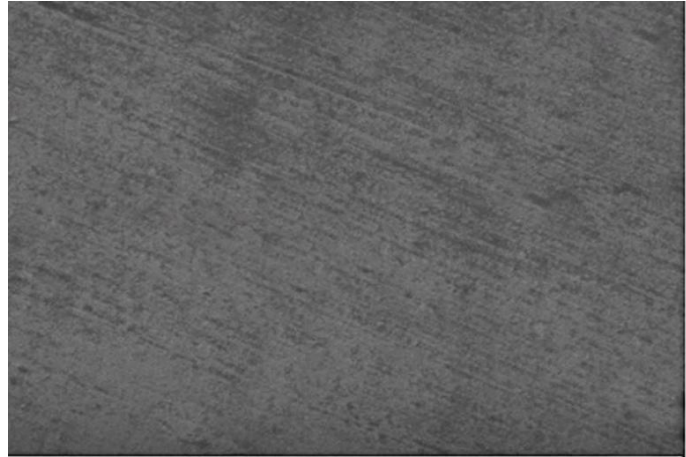
Fig5.1:Surface Morphology of bare FTO
