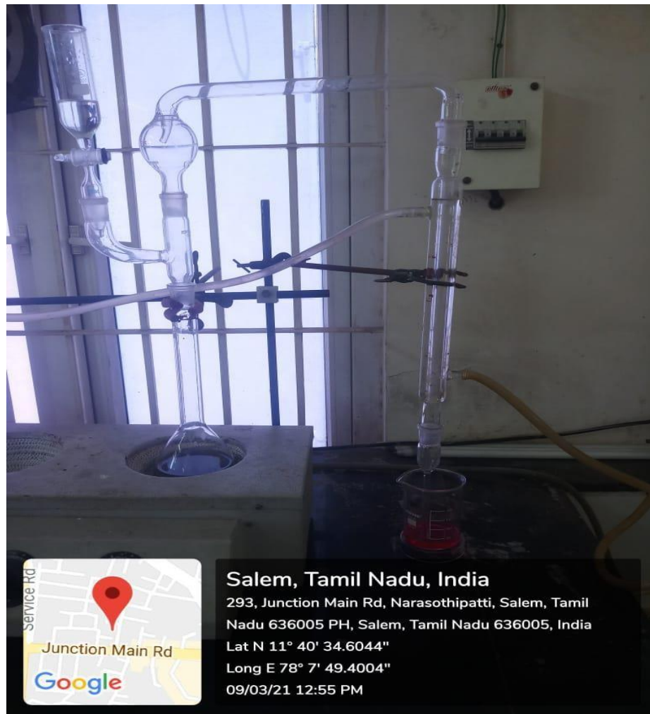
Fig 4.3.4 : Kjeldhal Distillation Unit used for Nitrogen content analysis
