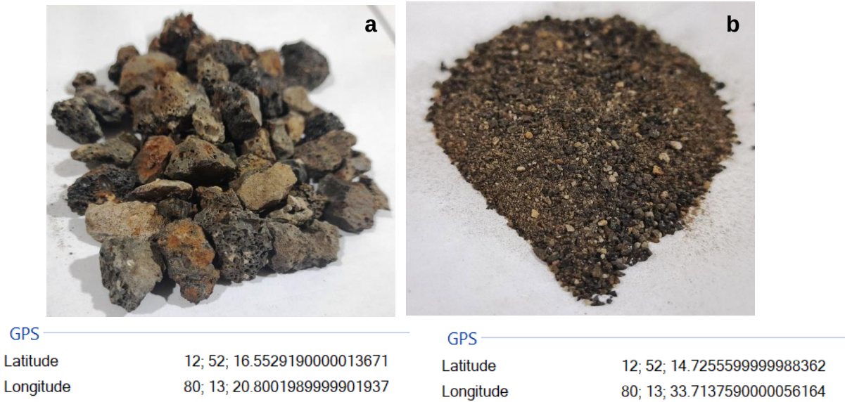
Figure 3.1: shows induction furnace (IF) steel slag (a) stone form; (b) powder form
