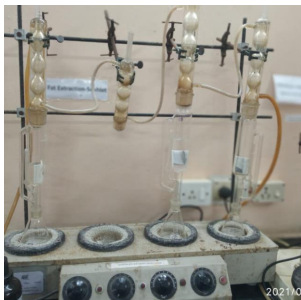
Figure 4.13 Soxhlet apparatus for fat extraction
