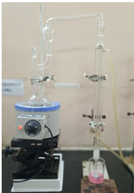
Figure 4.10 Kjeldahl apparatus setup for protein test
