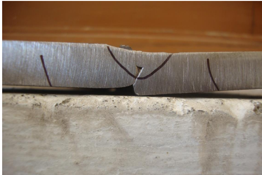
Fig. 5.1: View of test plate-1 (AMPS-140, VOLT-18, BEVEL-55)
