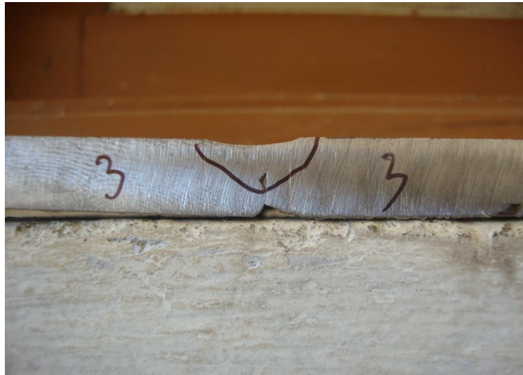
Fig. 5.3: View of test plate-3 (AMPS-140, VOLT-22, BEVEL-70)
