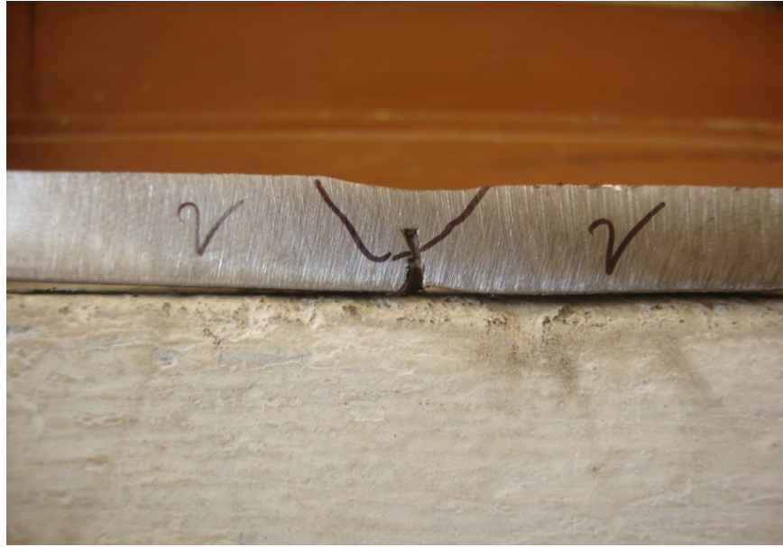
Fig. 5.2: View of test plate-2 (AMPS-140, VOLT-20, BEVEL-65)
