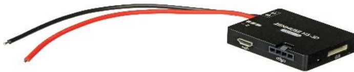
Fig. 4.18: Gimbal Controller Unit
