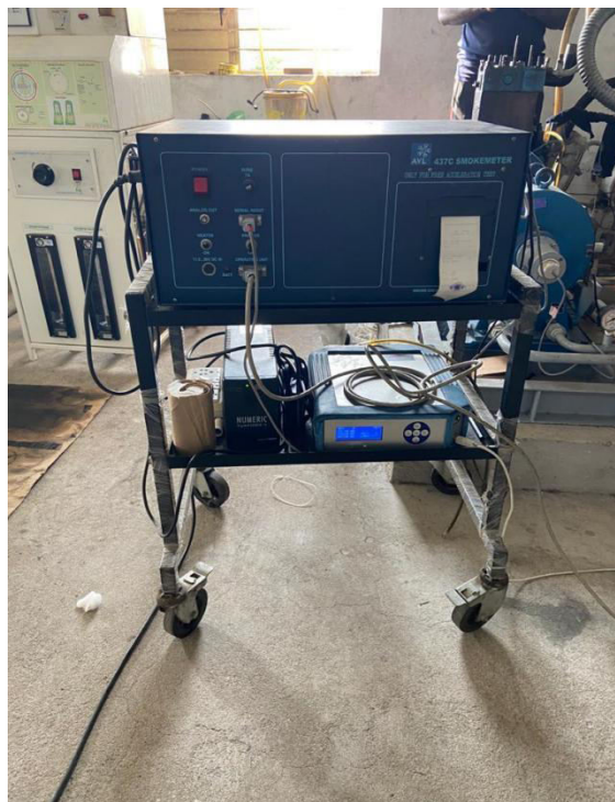
Fig: 4.8: Smoke meter and Gas Analyzer
