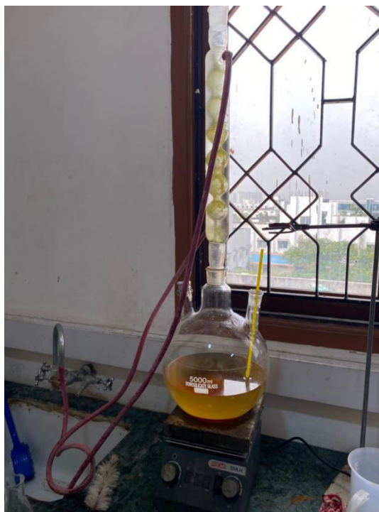
Fig: 4.3 : Separation of glycerin from Bio-diesel.
