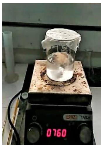
Fig: 4.4: Mixing of Catalyst with alcohol
