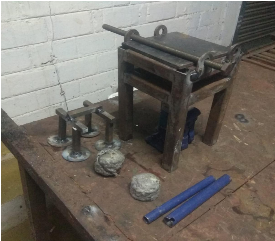
Fig 3.6: Developed Briquetting machine
