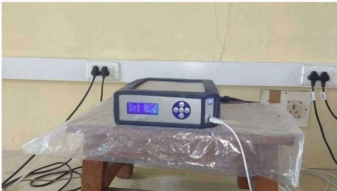
Figure 5.5 Five Gas Analyzer
