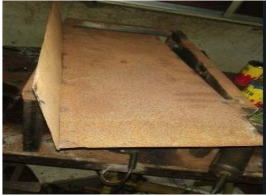
Fig 4.11 Fabrication Sheet cutting to cover upon the rectangular frame.
