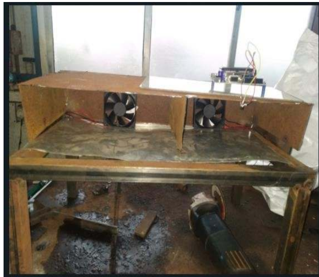
Fig 4.15 Fabrication Fully assembled cooling and heating box along with the Peltier module.
