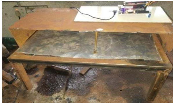
Fig 4.13 Fabrication Microcontroller with temperature showing LCD display is fixed to the frame.
