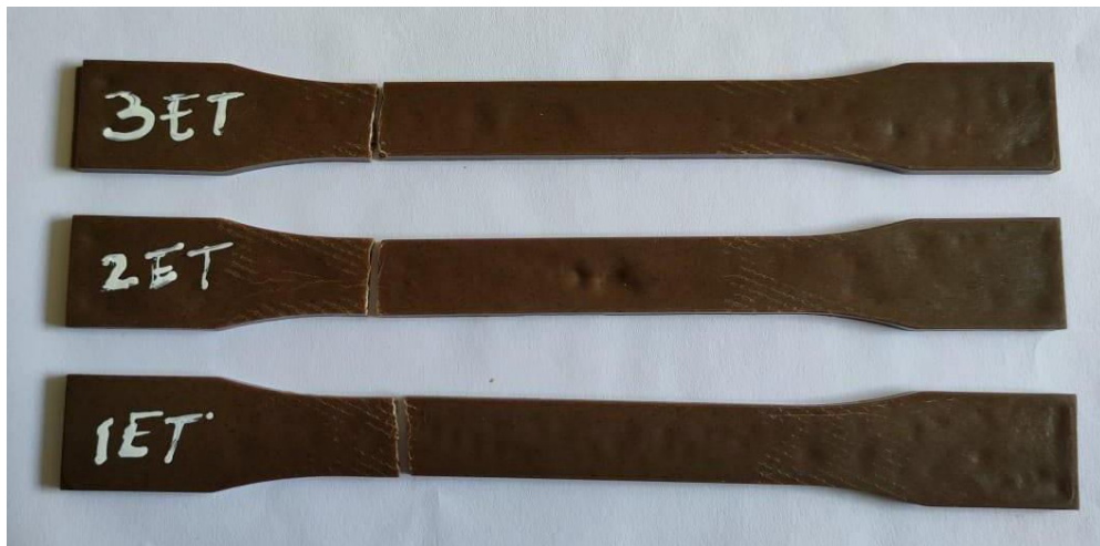
Fig:5.2 : Extrusion-injection moulded sample after tensile test.
