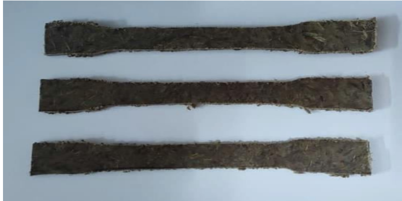
Fig:4.20 : Tensile samples by compression moulding
