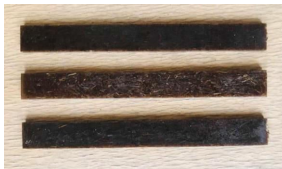
Fig:4.10 : Tensile samples by injection moulding
