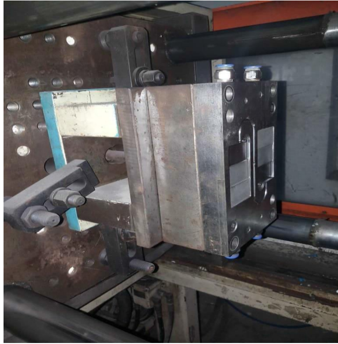
Fig:4.9 : Injecting the extruded mixture to molds
