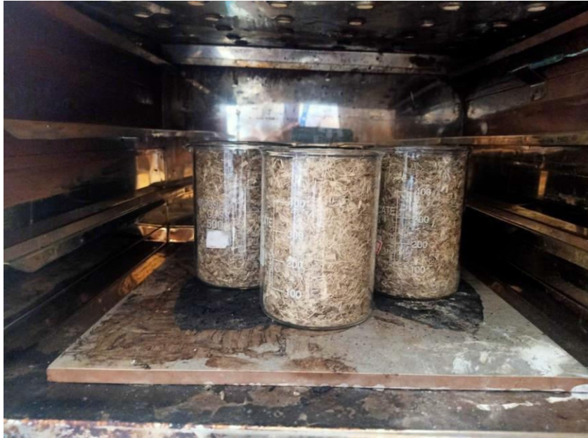
Fig:4.5 : Owen treatment at 100 0 C
