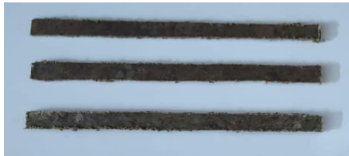
Fig:4.21 : Flexural samples by compression moulding
