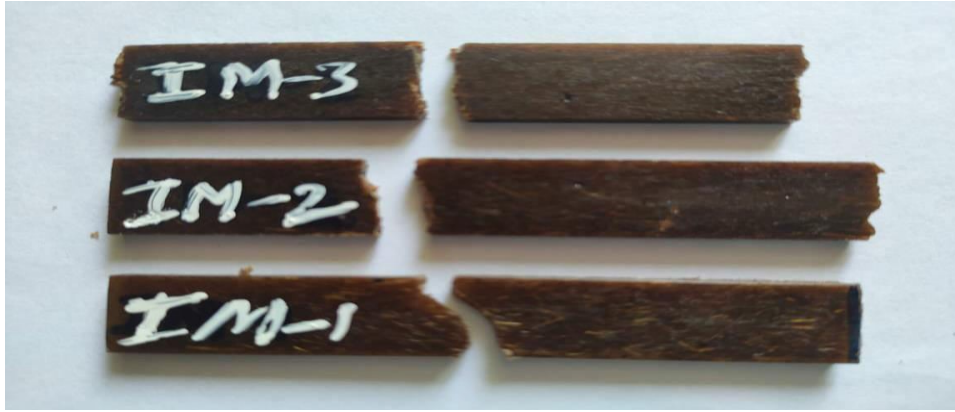
Fig:5.11 : injection moulded samples after Impact testing
