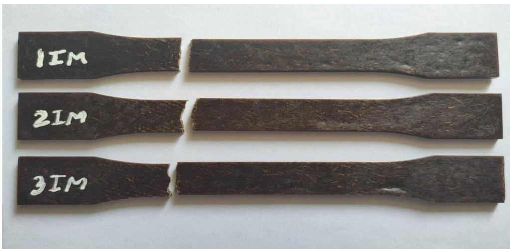
Fig:5.1 : injection moulded sample after tensile test
