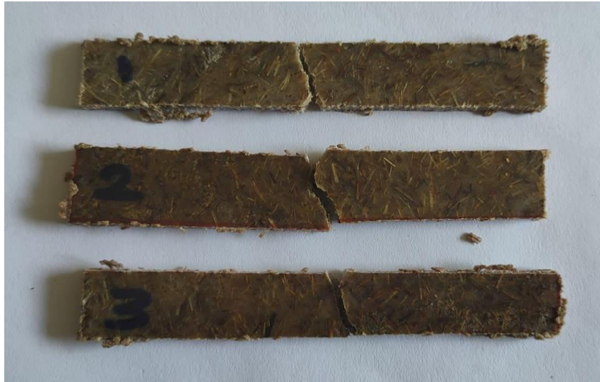
Fig:5.13 : Compression moulded samples after Impact testing
