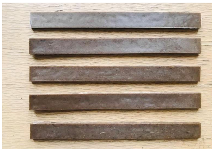
Fig:4.15 : Tensile samples by extrusion-injection moulding
