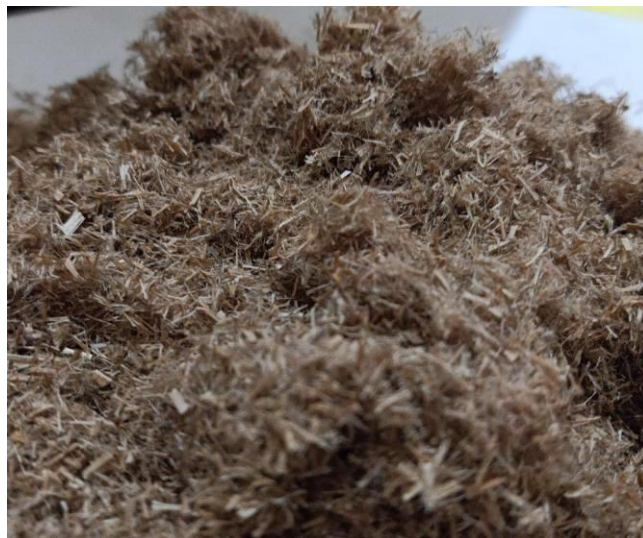
Fig:4.4 : The fiber that has been cut by scissors
