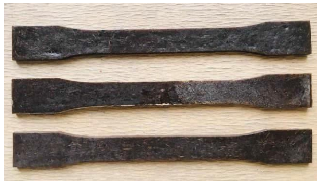
Fig:4.10 : Tensile samples by injection moulding
