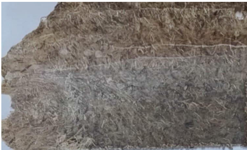
Fig:4.19 : Plate that has been made through compression moulding
