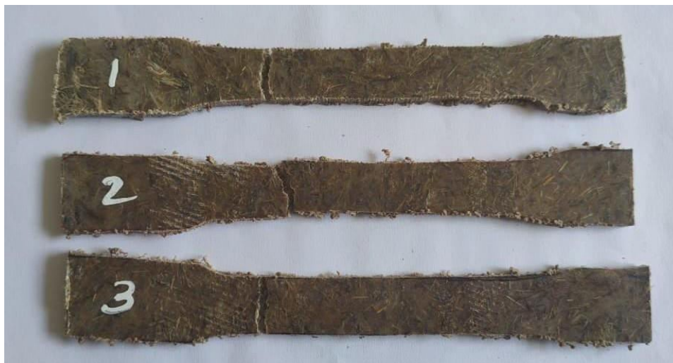
Fig:5.3 : Compression moulded sample after tensile test.
