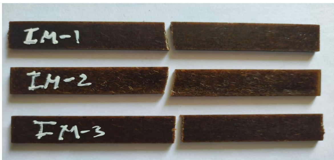
Fig:5.6 : Injection moulded sample after flexural test.
