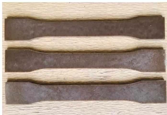
Fig:4.15 : Tensile samples by extrusion-injection moulding
