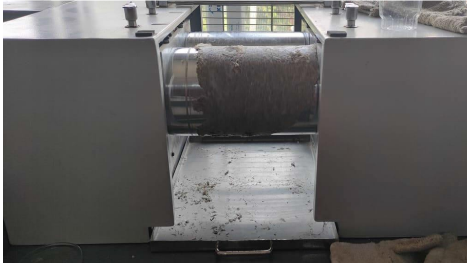
Fig:4.18 : Fiber grinding along with PLA
