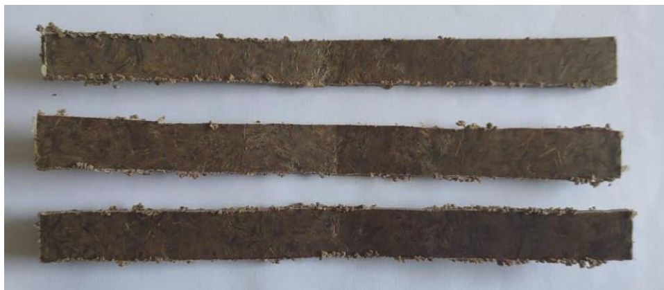
Fig:5.8 : Compression moulded sample after flexural test
