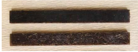
Fig:4.12 : Impact samples by injection moulding
