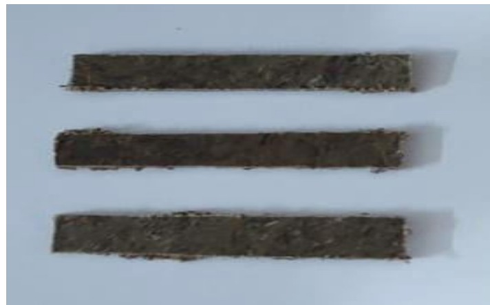
Fig:4.22 : impact test samples by compression moulding
