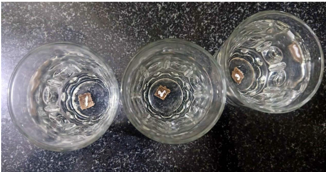
Fig:4.28 : Samples that are being tested for water absorption
