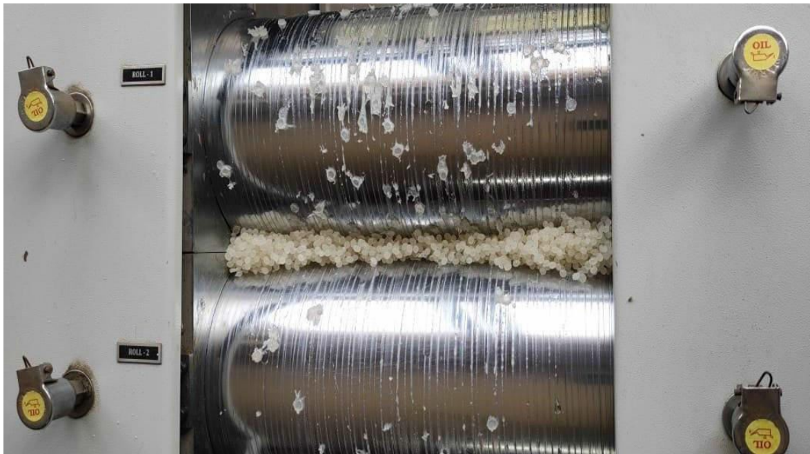
Fig:4.17 : Grinding PLA with 2 roll milling
