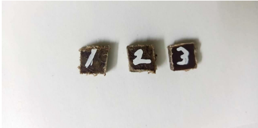
Fig:4.27 : 1*1 cm samples for water absorption test
