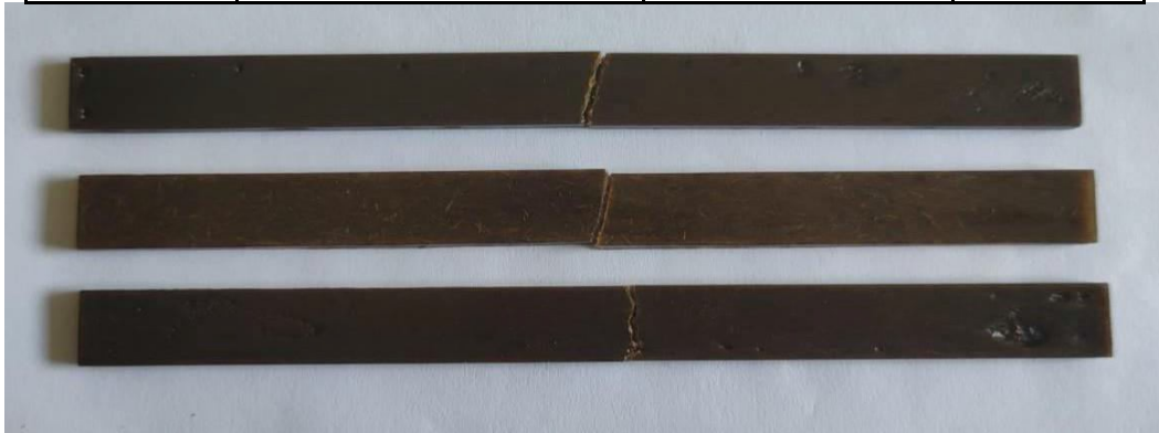
Fig:5.7 : Extrusion-Injection moulded sample after flexural test
