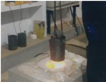
Figure 4.3 Placing Crucible with Mg in Furnace
