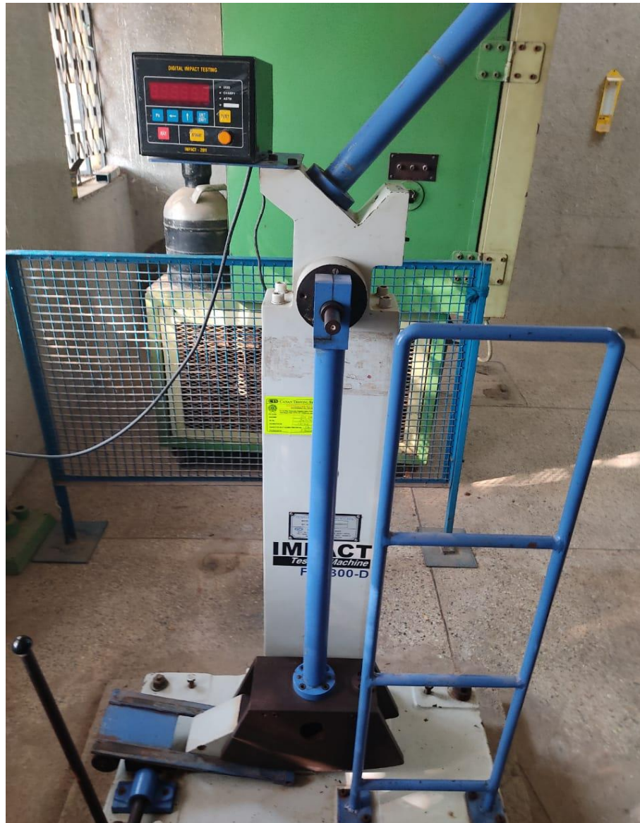
Fig 5.3: Impact testing machine
