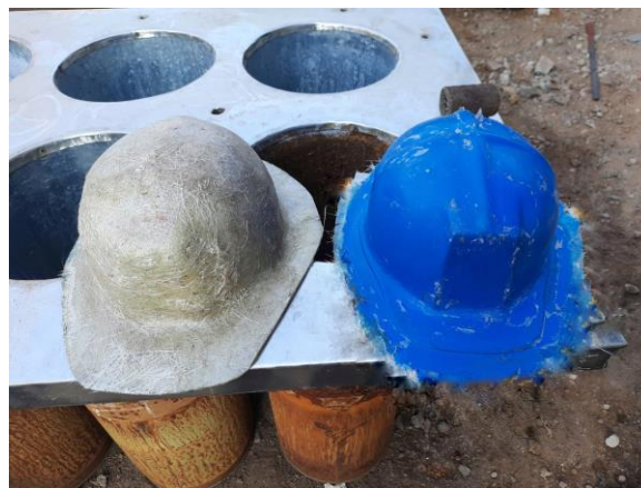
Fig 4.8: After separating helmet from mould
