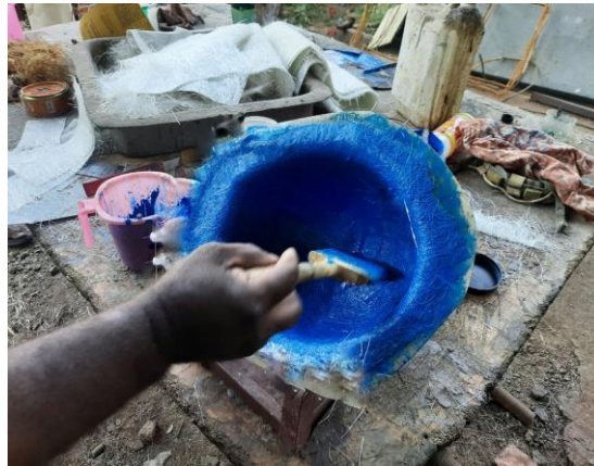
Fig 4.7: Sticking fiber into the mould
