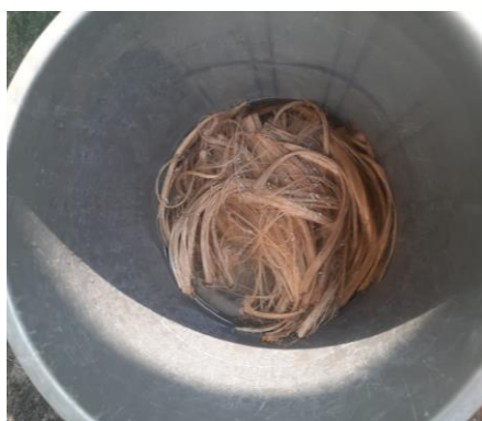
(b) Fibers in NaOH solution
