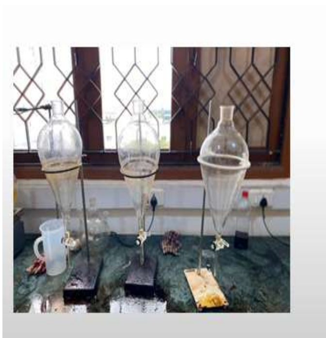
Fig: 4.3: Transesterification process.
