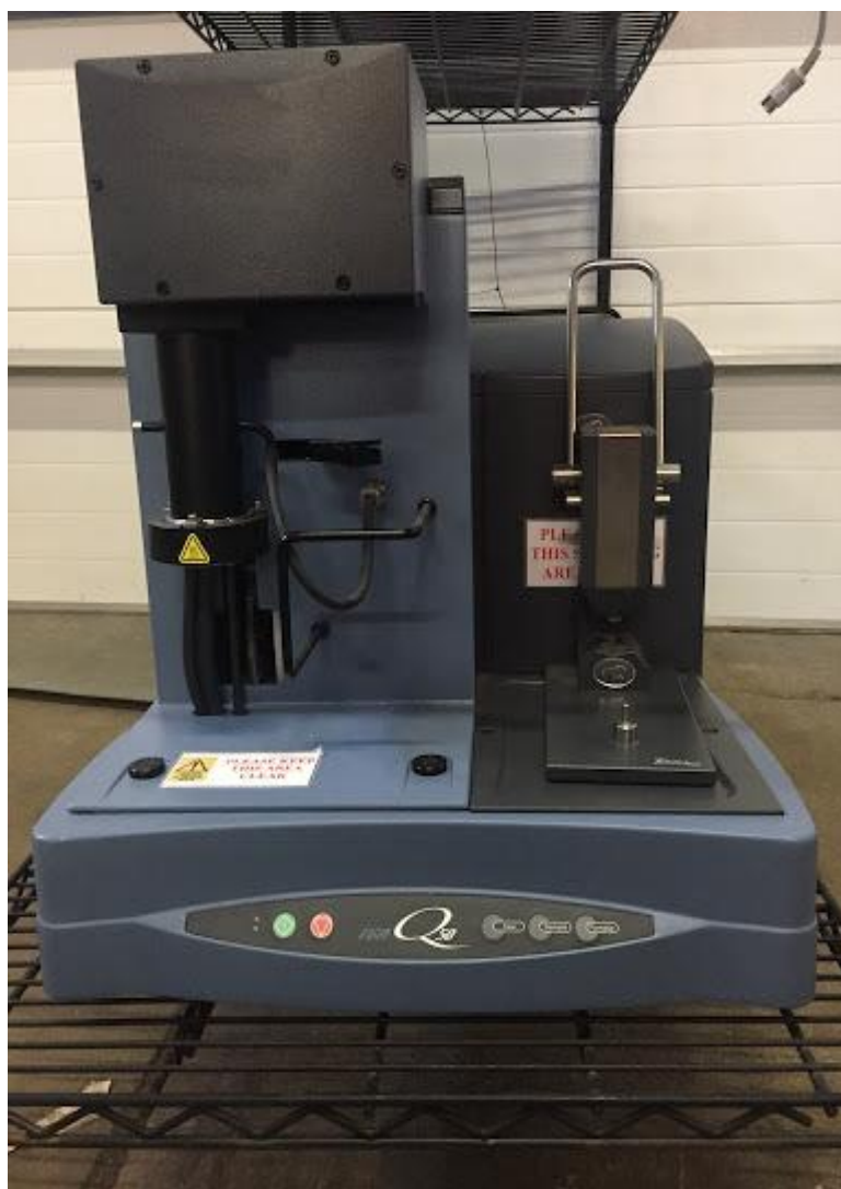
Fig:4.10 : TGA equipment
